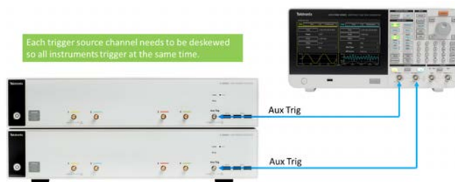
Synchronize multiple instrument channels within 200 ps using manual deskew and the Aux Trigger input
