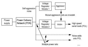
The image shows a multi-rail example of the effect of noise with various points of loads (POL) such as DDR memory, PCIe, etc.
