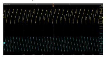
Perform this measurement for a single cycle within an acquisition or over every cycle within an acquisition (Cycle Mode). Synchronize cycles based on a power rail signal or another signal in the system. Cycle-by-cycle measurements are analyzed using statistics, histograms, or plots. Bandwidth limit capability enables designers to analyze the ripple numbers at different bandwidths.
