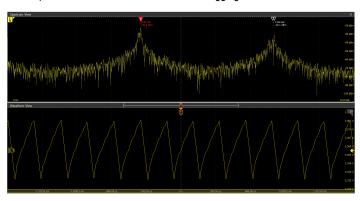
Analyze cycle-by-cycle by selecting a PWM clock (if available) and view peakpeak and RMS values for each ripple cycle. This gives statistics for all of the cycles within an acquisition. Bandwidth limit capability enables designers to analyze the ripple numbers at different bandwidths.
