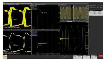
The image shows improvement in PSIJ results after removing the jitter which was added by the power rail source
