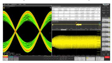
For instance, a SI (Signal Integrity) engineer can measure POL (Point of Load) powering the clock and observe the eye diagram where it is clean and opens up. If the eye diagram is not clean and if there are spurs from POL, then the PI (Power Integrity) engineer can work to modify their power supply design to get better sensitivity. This makes SI engineer see the improvement on the HSS load.
