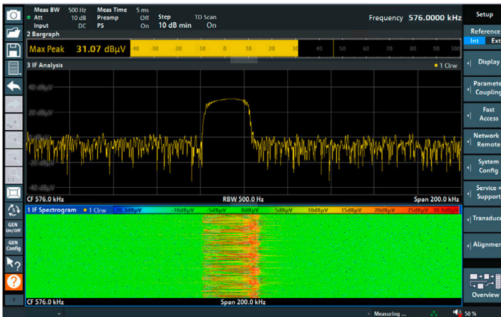
Analysis of the emissions of an LED lamp at 576 kHz using bargraph display in combination with IF spectrum and spectrogram function. The dynamic behavior of the signal, especially in the range of 560 kHz to 585 kHz, is clearly visible.
