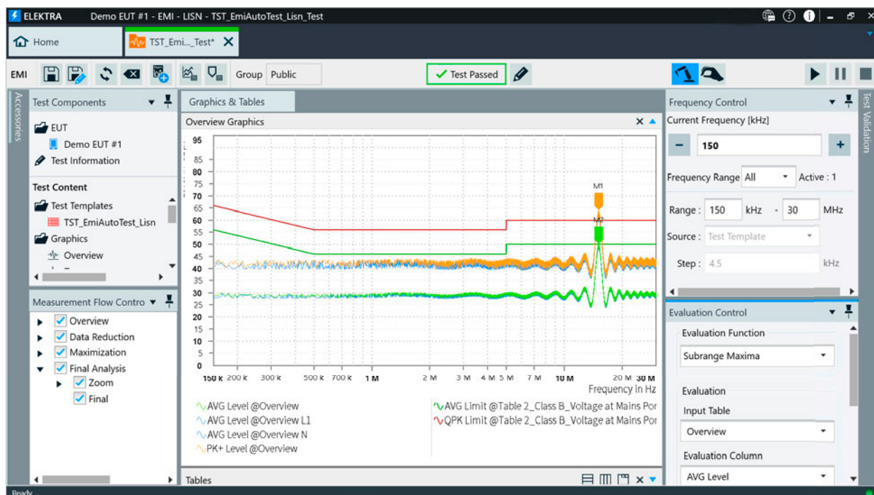
Automated EMI measurement with R&S®ELEKTRA.
