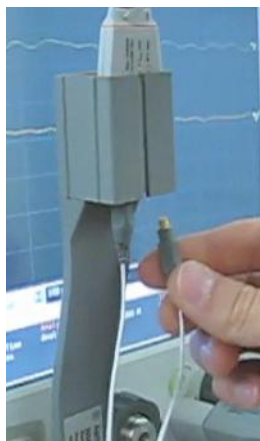
Figure 79 Connect the Head to the Probe
