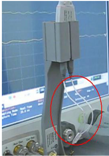
Figure 80 Positioning the Probe Head Wires
