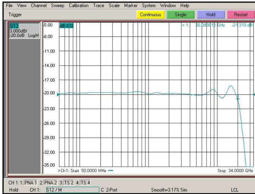
Figure 107 De-Embedded V_{out}/V_{in} Response of the Probe
