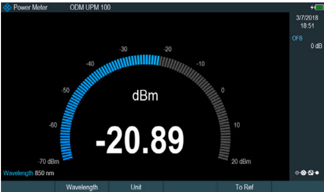
Optical power measurement with optical power sensor.
