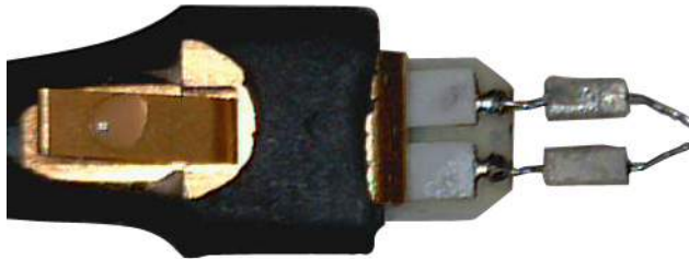
Figure 22 Proper Position of Resistors
