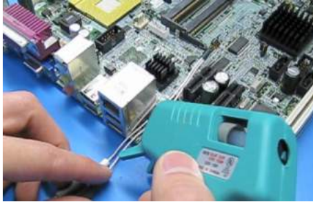
Figure 48 Using low-temperature hot glue to secure a probe head
