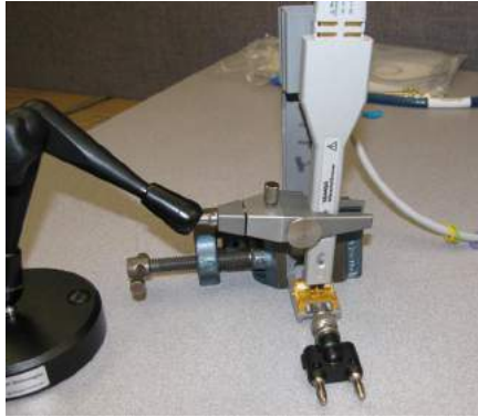
Figure 72 Setup for Measuring Input Resistance for Browser Probe Head
