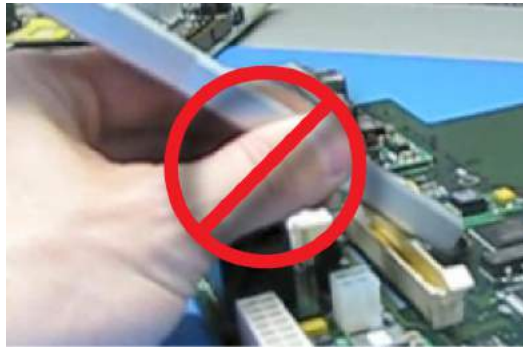
Figure 16 Improper Probe Handling
