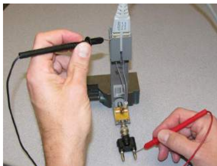
Figure 71 Measuring the single-ended input resistance of a ZIF or solder-in probe head
