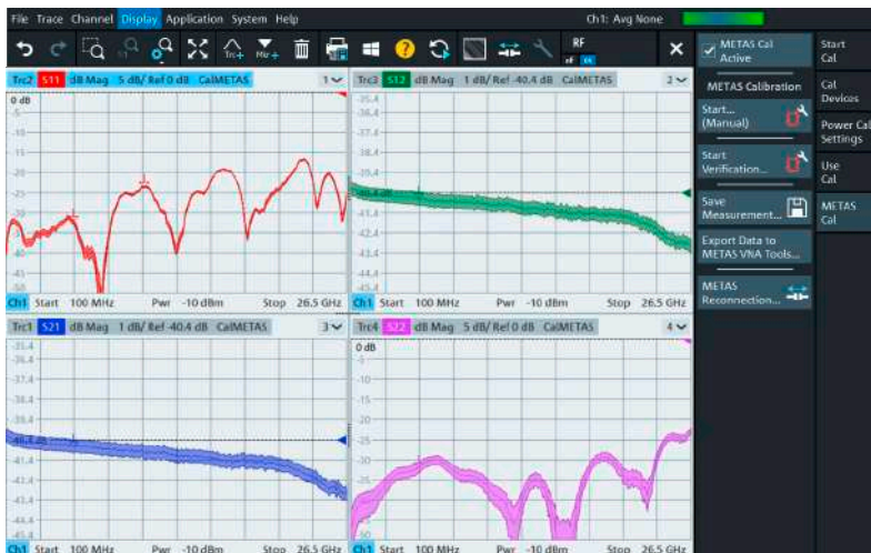
Real-time S-parameter measurements with uncertainty bands
