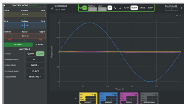
Embedded WAVEFORM GENERATOR and 4-channel OSCILLOSCOPE
