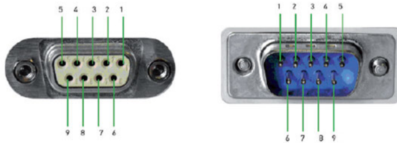
Figure A-2: RS232 Pin Assignment
