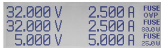
Figure 4-6: Overvoltage protection (example R&S HMP2030)
