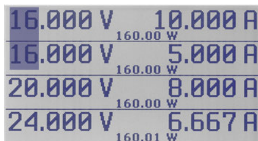
Figure 4-3: Setting the same voltage for two channels with the tracking function
