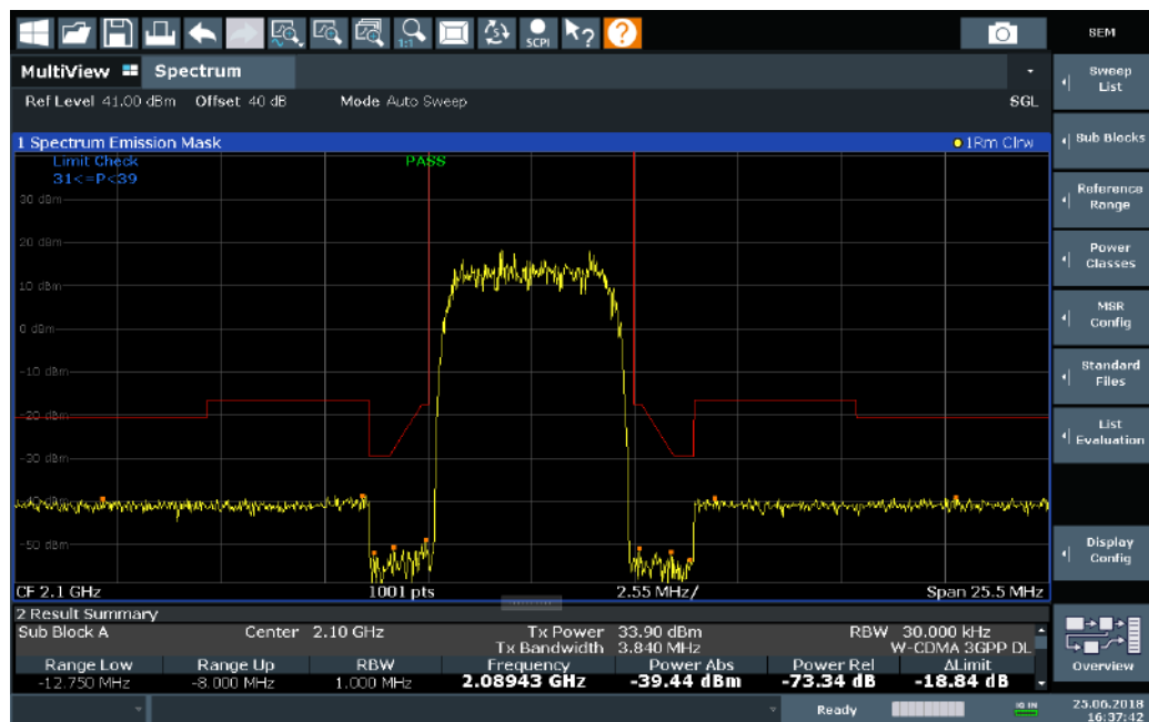
Figure 5-42: Detected peak display in SEM measurement
