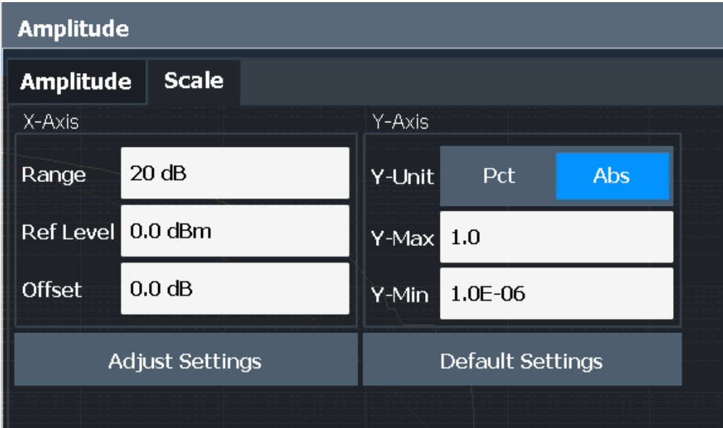
Figure 5-48: Scale settings for CCDF diagram
