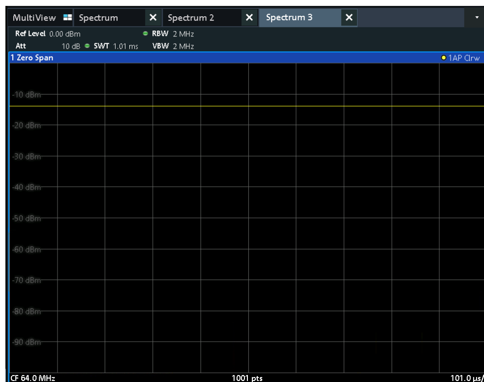
Figure 3-11: Time domain display of the calibration signal
