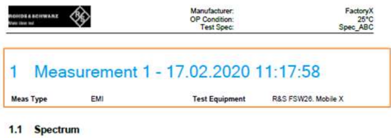
Figure 9-4: Example for measurement-specific information in a test report
