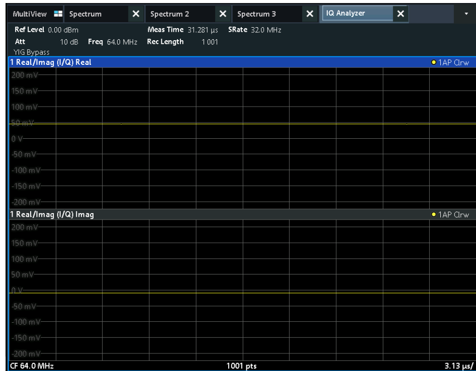
Figure 3-12: Inserting a Real/Imag diagram for I/Q analysis
