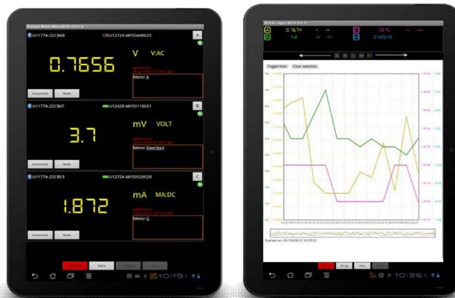
Figure 3. Once connected to any HH DMM via Bluetooth adapter you are able to log and view measurements graphically from smart phones and tablets.
