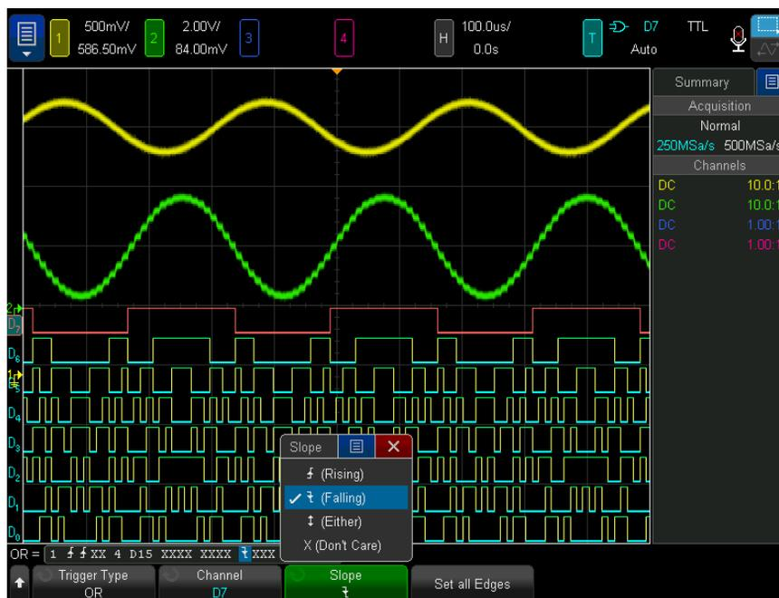
If all channels in the OR trigger are set to don't care, the oscilloscope will not trigger.
