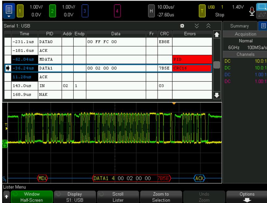
In addition to the standard Time column, the USB 2.0 Lister contains these columns:
