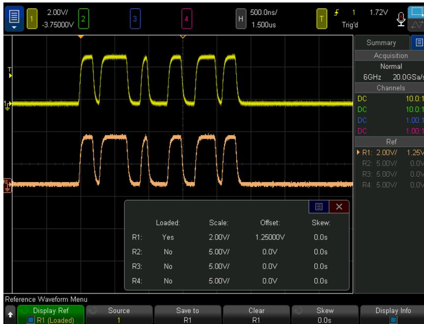
Reference waveforms are always drawn as vectors (that is, lines between waveform data points) and may look different than waveforms drawn as dots (if that option is available in your oscilloscope).
