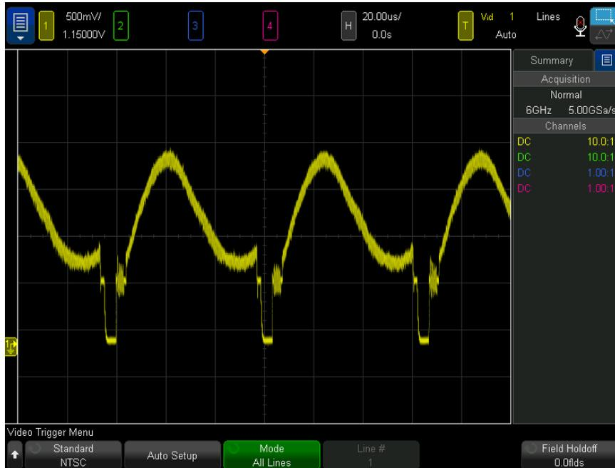
**Figure 30** Triggering on All Lines
