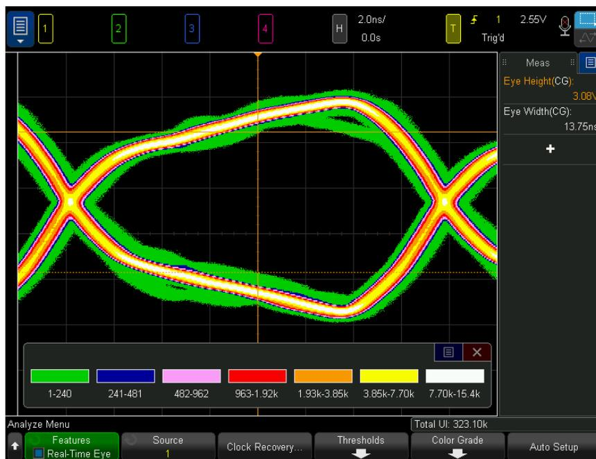
**10** To stop real-time eye analysis acquisitions, press the **[Stop]** front panel key.
