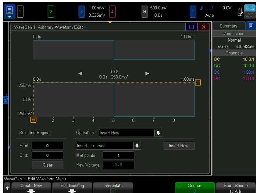
When you open the Edit Waveform Menu, you see the existing arbitrary waveform definition. The voltage and time period you see in the diagram are the bounding parameters – they come from the frequency and amplitude settings in the main Waveform Generator Menu.
