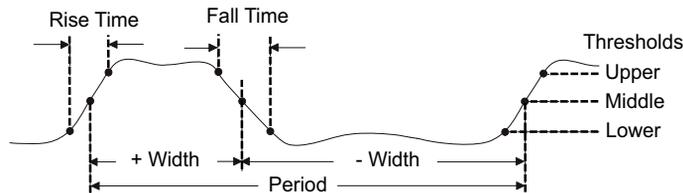
The default lower, middle, and upper measurement thresholds are 10%, 50%, and 90% between Top and Base values. See "**Measurement Thresholds**" on page 283 for other percentage threshold and absolute value threshold settings.
