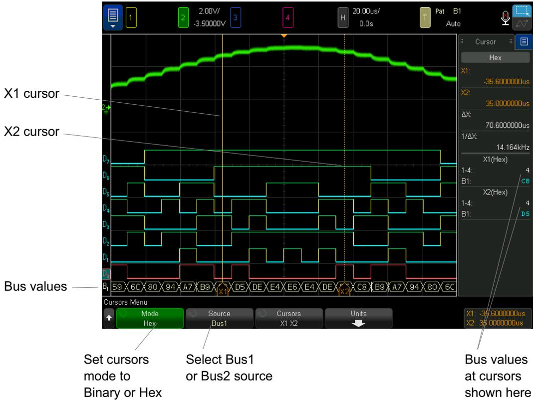
**Bus values are displayed when using Pattern trigger**
