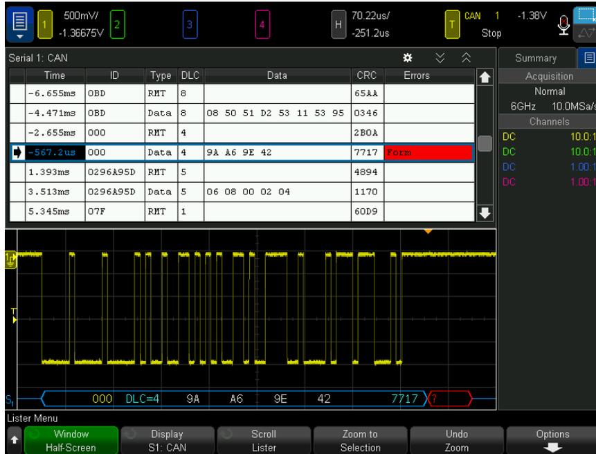
In addition to the standard Time column, the CAN Lister contains these columns:
