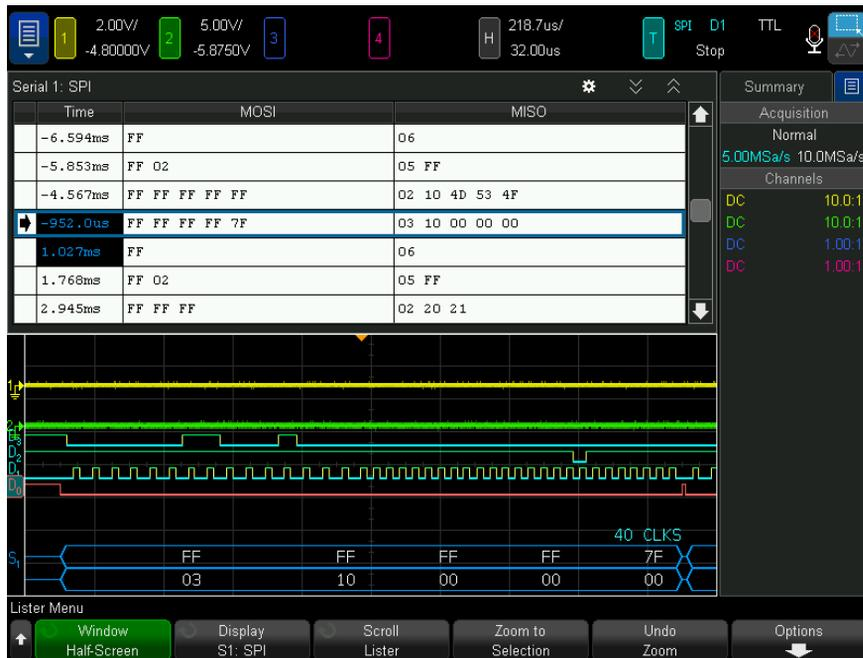
In addition to the standard Time column, the SPI Lister contains these columns:
