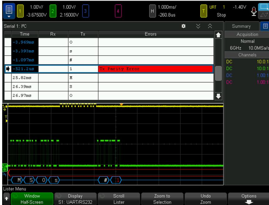
In addition to the standard Time column, the UART/RS232 Lister contains these columns:
