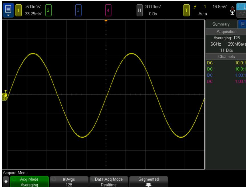
**Figure 41** 128 Averages used to reduce random noise
