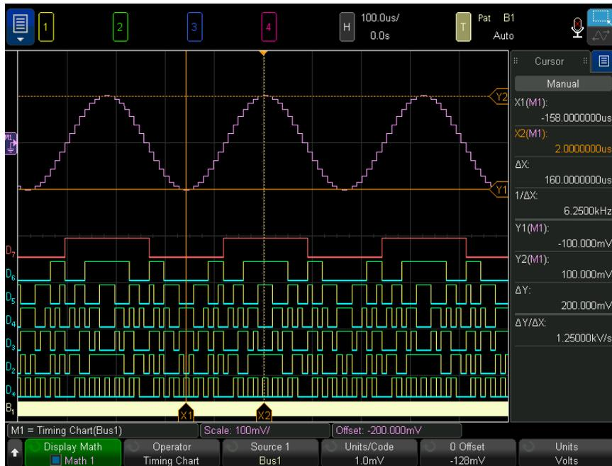
**Figure 19** Example of Chart Logic Bus Timing
