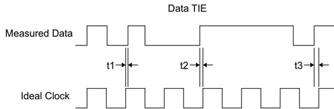
The measurement is made on all the cycles of the waveform. Even in Zoom mode, all the cycles of the waveform in the Main window will be measured.
