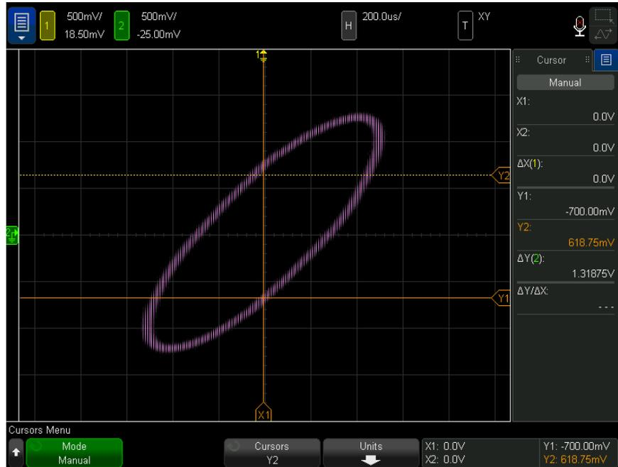
**Figure 4** Phase difference measurements, automatic and using cursors
