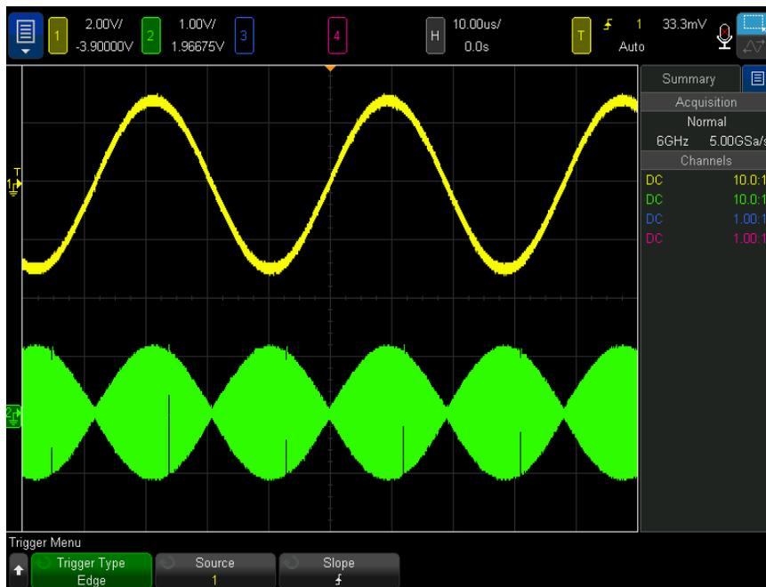
**Figure 27** Amplitude Modulation Shown at 100% Intensity
