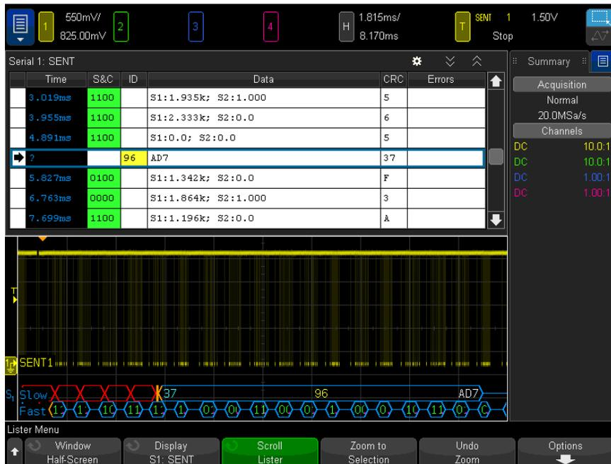
Each Fast or Slow Channel message is represented on its own row. The start time of Slow Channel messages determines their order relative to the Fast Channel messages. Therefore, a Slow Channel message appears before most of the Fast Channel messages that it was built from. This is due to the "Time" column holding the start time of a packet.
