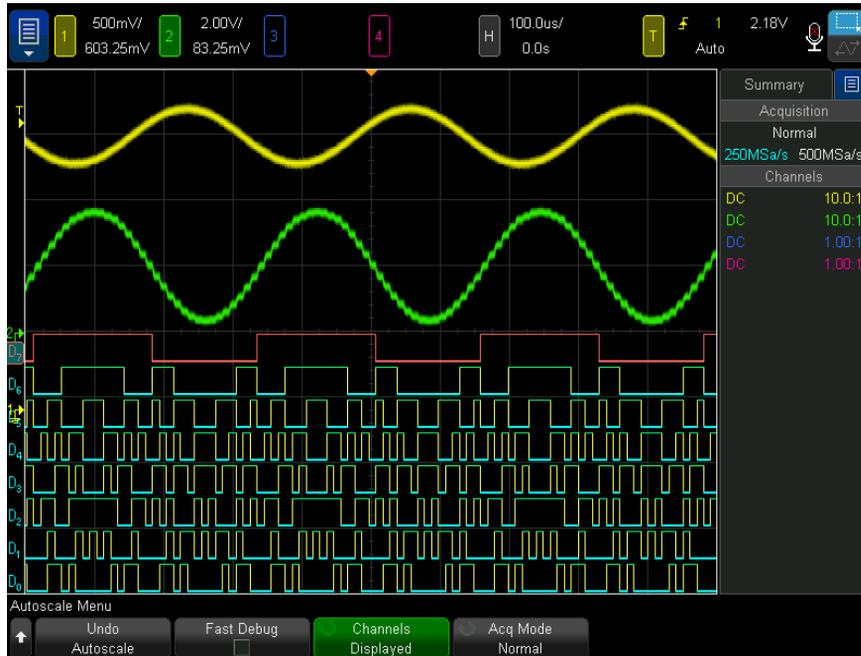
**Figure 22** Example: Autoscale of digital channels (MSO models only)
