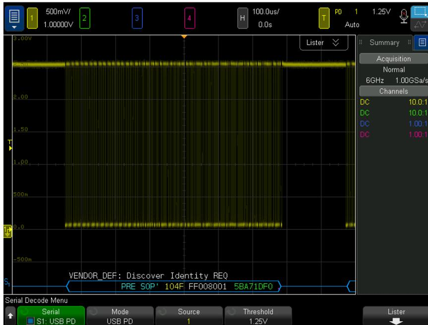
The USB PD decode is displayed as a single bus, with one decode line positioned at the bottom of the waveform area, time-aligned with the associated physical signal. Above the decode line is abbreviated symbolic decode information, shown in white, that describes the header's port power role (bit 8), port data role (bit 5), and message type (bits 4-0).
