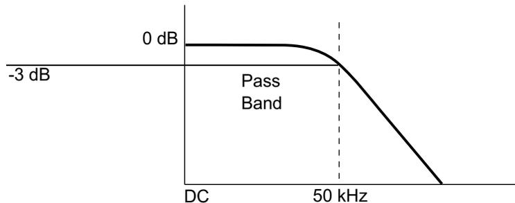
You can use HF Reject to remove high-frequency noise, such as AM or FM broadcast stations or noise from fast system clocks, from the trigger path.
