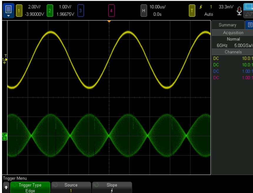
**Figure 28** Amplitude Modulation Shown at 40% Intensity
