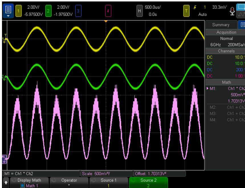
**Figure 6** Example of Multiply Channel 1 by Channel 2
