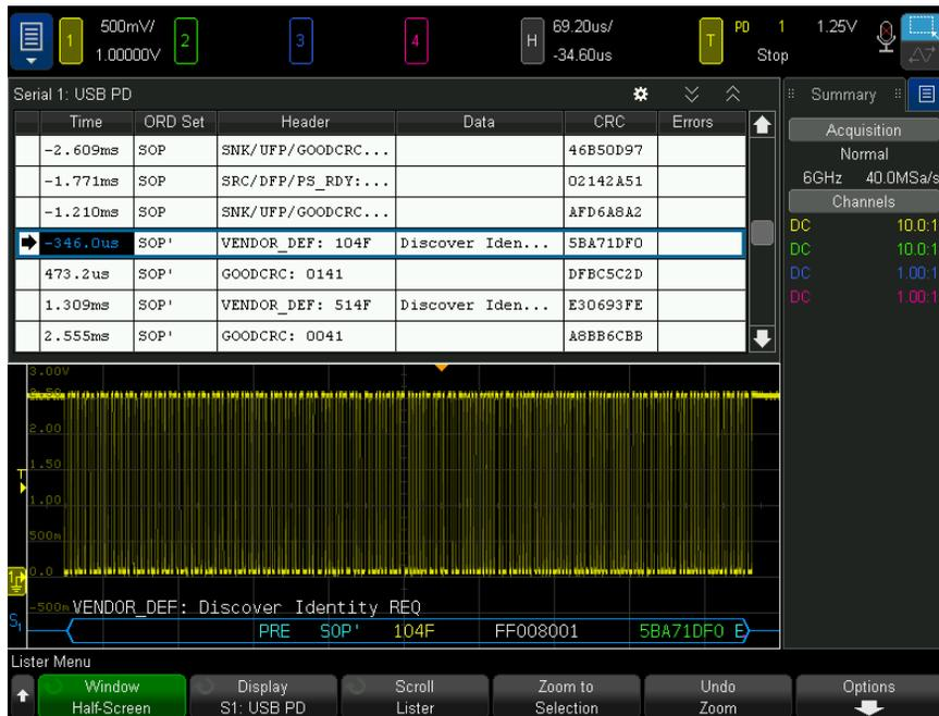
In addition to the standard Time column, the USB PD Lister contains these columns:
