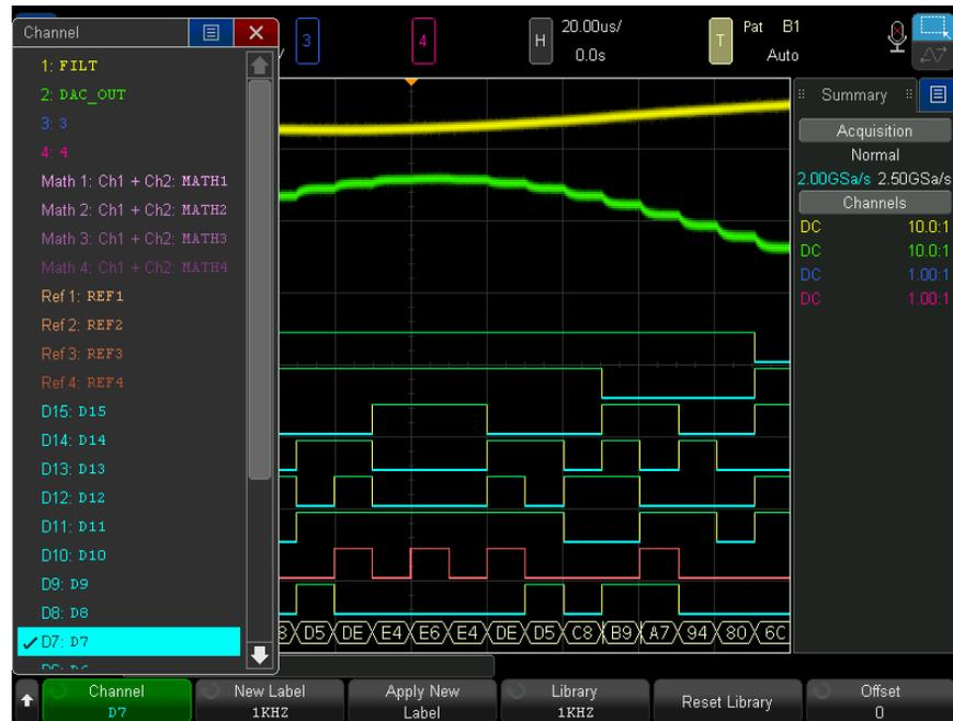
The figure above shows the list of channels and their default labels. The channel does not have to be turned on to have a label assigned to it.
