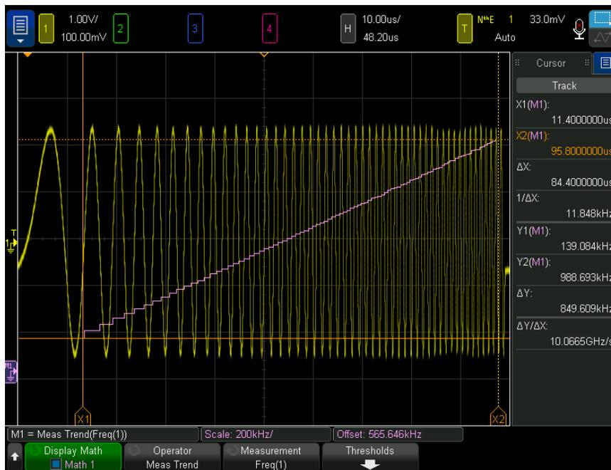
**Figure 18** Example of Measurement Trend
