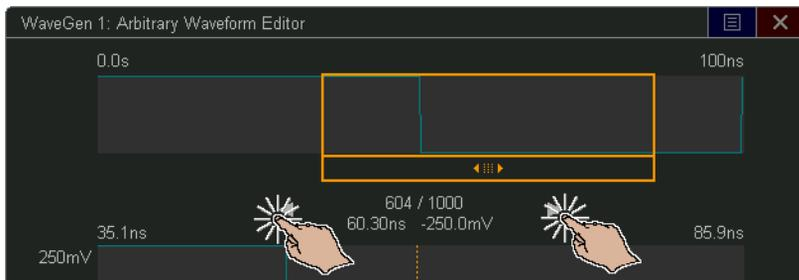
To adjust the value of a point, drag the voltage level handle up or down:
