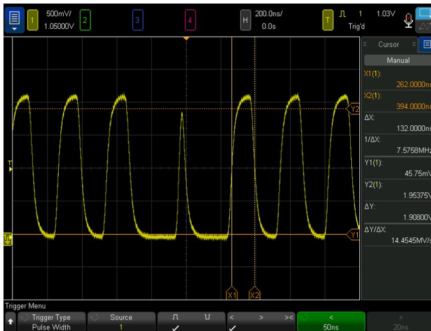
**Figure 45** Measuring pulse width with cursors
