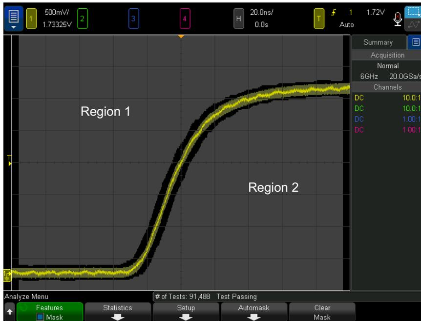
Up to 8 regions can be defined for a mask. They can be numbered 1-8. They can appear in any order in the .msk file. The numbering of the regions must go from top to bottom, left to right.
