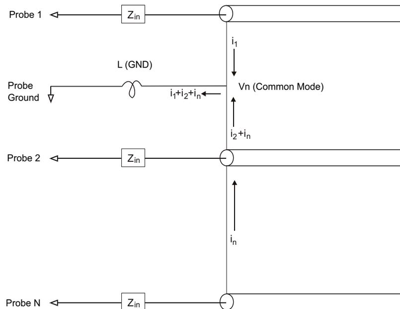
**Figure 26** Common Mode Input Voltage Model
