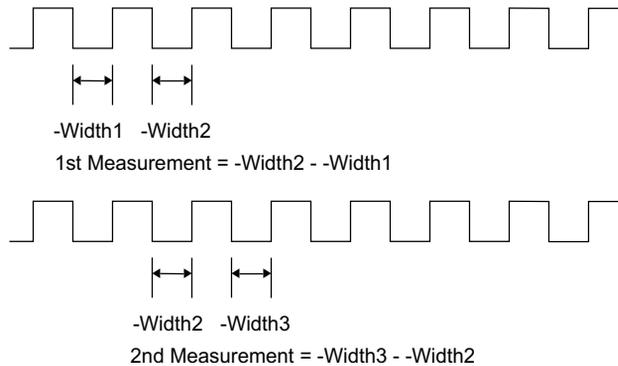
All of the measurement results are used to compute the statistics. The statistics are the values accumulated over all of the trigger cycles that have occurred.
