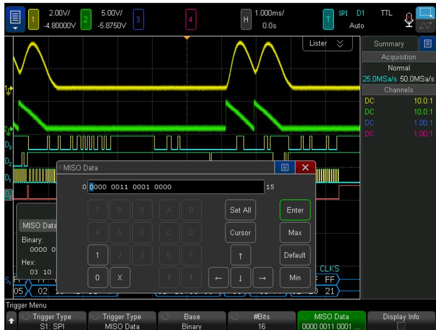
The data value is left-justified in the frame when setting up the trigger. If the base is Hex, the first digit represents the first 4 bits after the start of frame, continuing with the remaining digits in the data value.
