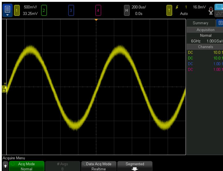
**Figure 40** Random noise on the displayed waveform
