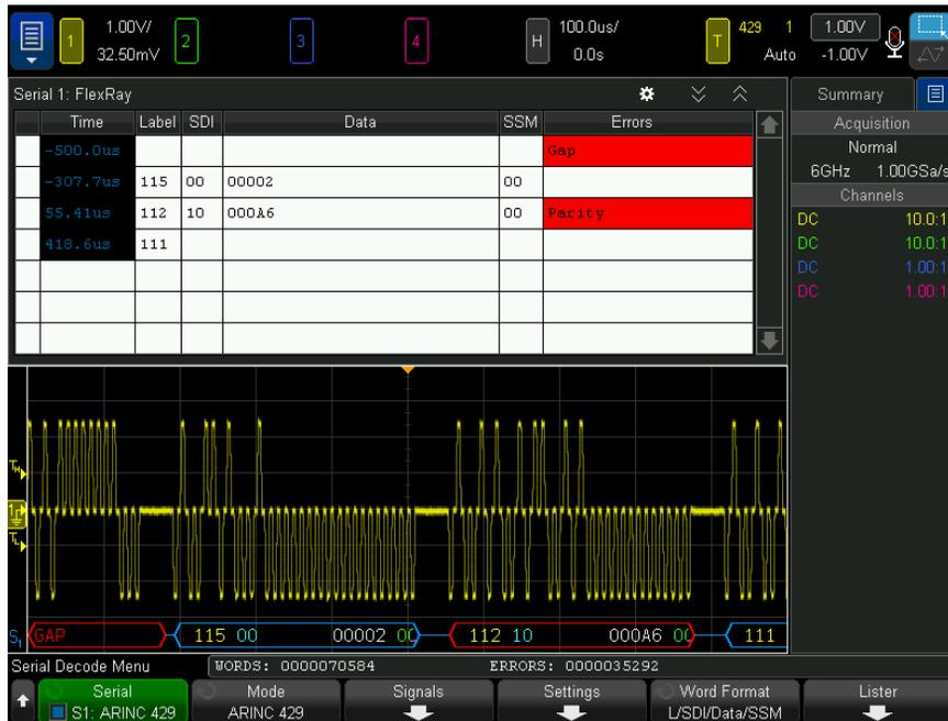
Depending on the selected word decode format, the ARINC 429 decode display is color coded as follows:
