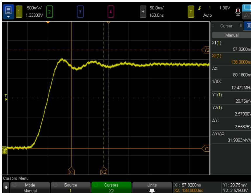
**Figure 43** Cursors measure frequency of pulse ringing
