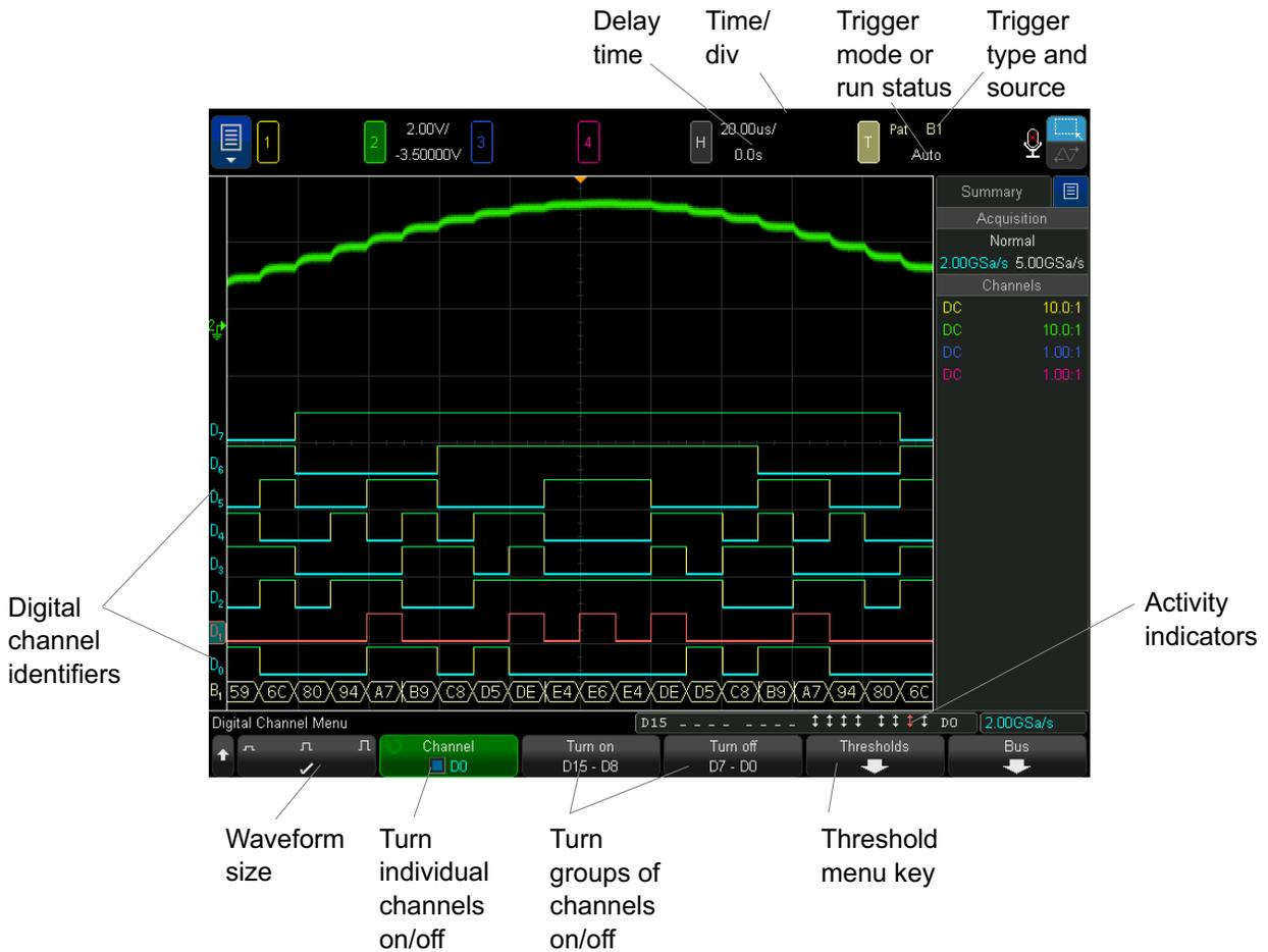
**Activity indicator** When any digital channels are turned on, an activity indicator is displayed in the status line at the bottom of the display. A digital channel can be always high (■), always low (■), or actively toggling logic states (↕).
