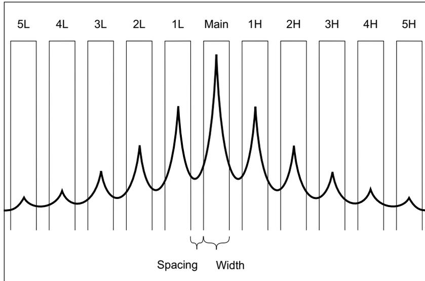
The sideband used for the measurement is selected with the Channel Select parameter. You can select the first through fifth sidebands above or below the main range (1H through 5H above and 1L through 5L below). The full sideband must be in the graticule to be measured. Otherwise, the measurement results will be "Incomplete".
