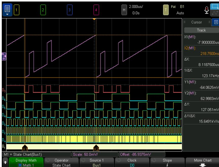
**Figure 20** Example of Chart Logic Bus State
