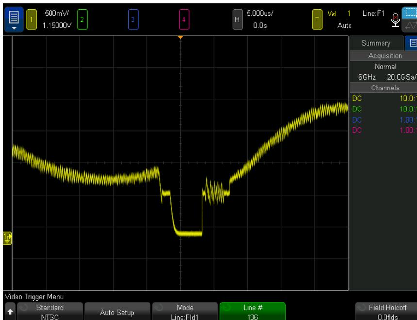
**Figure 29** Example: Triggering on Line 136
