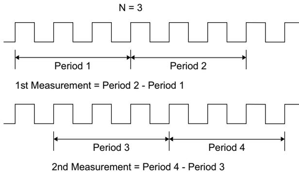
Once all of the groups of cycles of the waveform are measured, the statistics are calculated. The statistics are the values accumulated over all of the trigger cycles that have occurred.
