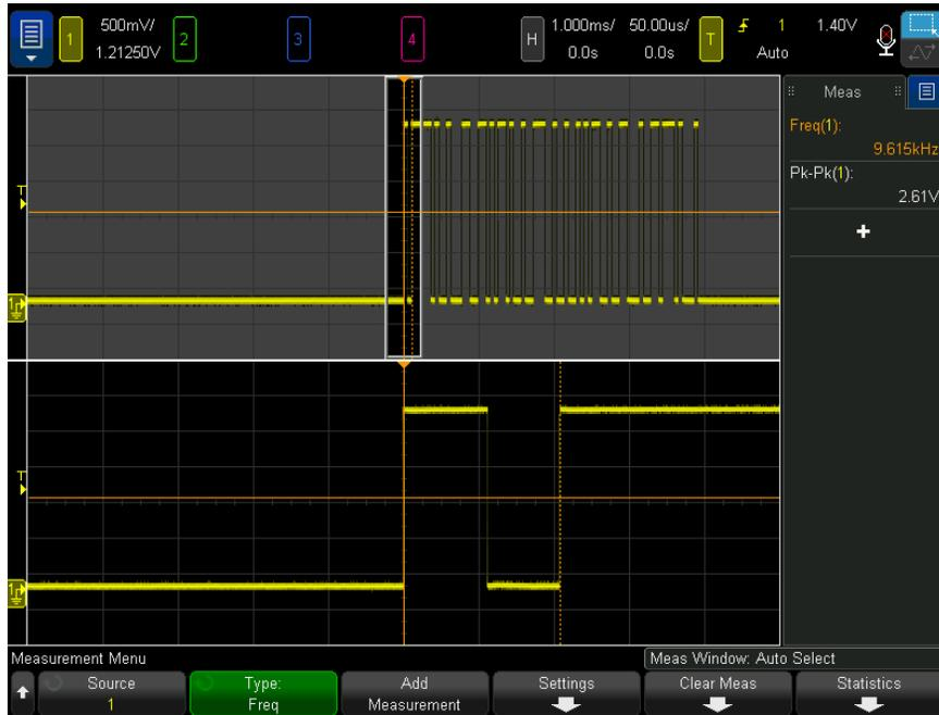
**Figure 50** Isolating an event for Frequency measurement
