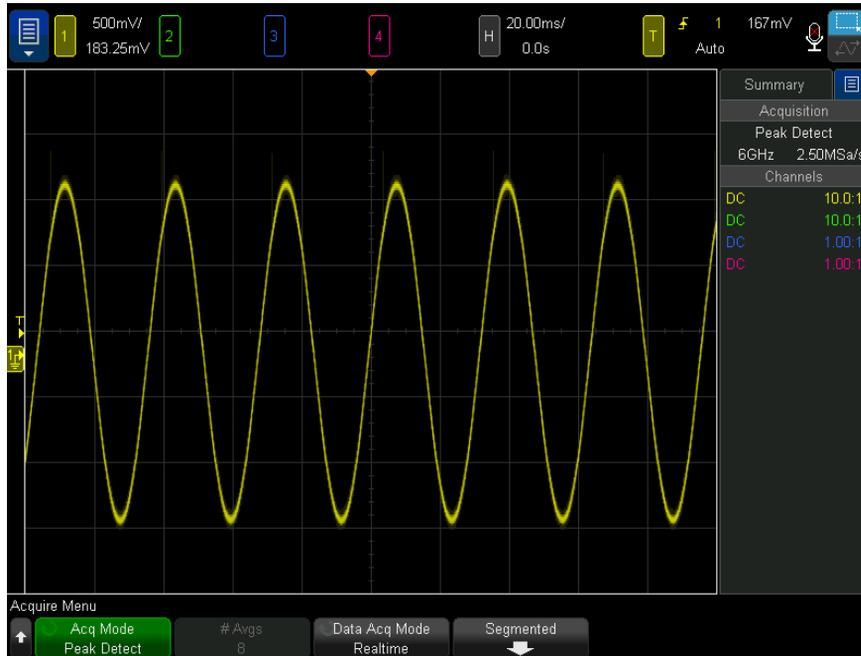
**Figure 39** Sine With Glitch, Peak Detect Mode
