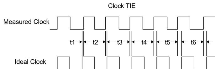
The measurement is made on all the cycles of the waveform. Even in Zoom mode, all the cycles of the waveform in the Main window will be measured.
