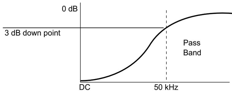
Low frequency reject removes any unwanted low frequency components from a trigger waveform, such as power line frequencies, etc., that can interfere with proper triggering.
