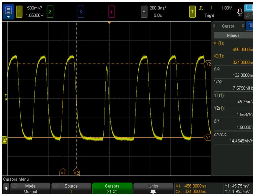
**Figure 46** Moving the cursors together to check pulse width variations
