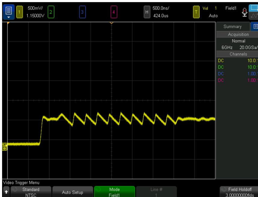
**Figure 34** Using Field Holdoff to Synchronize to Color Field 1 or 3 (Field 1 mode)
