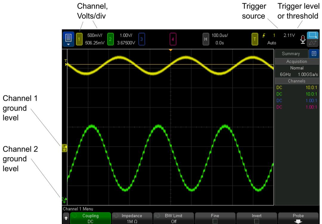
The ground level of the signal for each displayed analog channel is identified by the position of the
