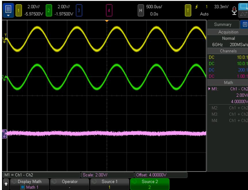
**Figure 5** Example of Subtract Channel 2 from Channel 1
