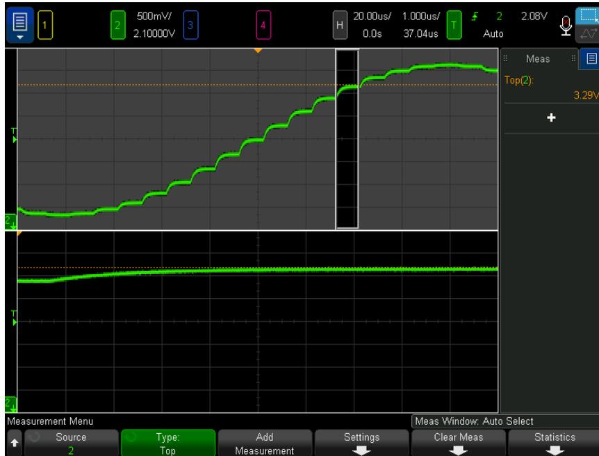
**Figure 48** Isolating area for Top measurement
