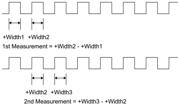
All of the measurement results are used to compute the statistics. The statistics are the values accumulated over all of the trigger cycles that have occurred.
