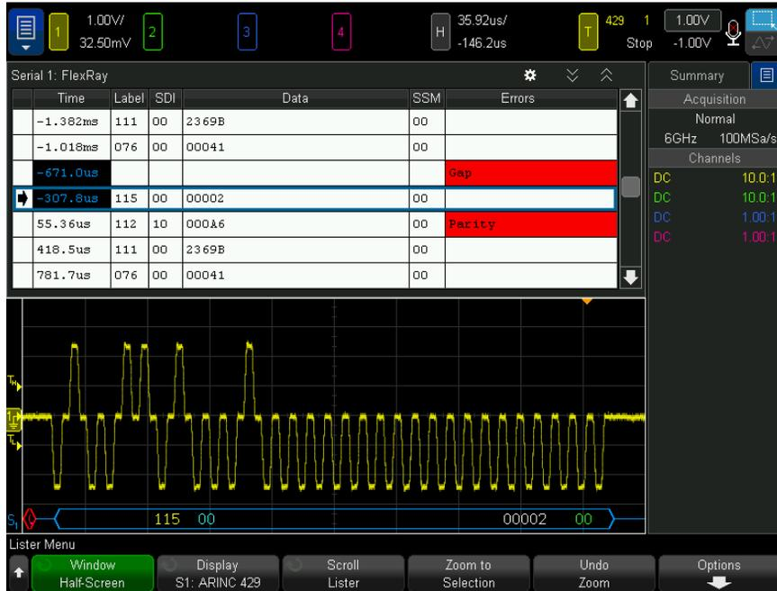
In addition to the standard Time column, the ARINC 429 Lister contains these columns:
