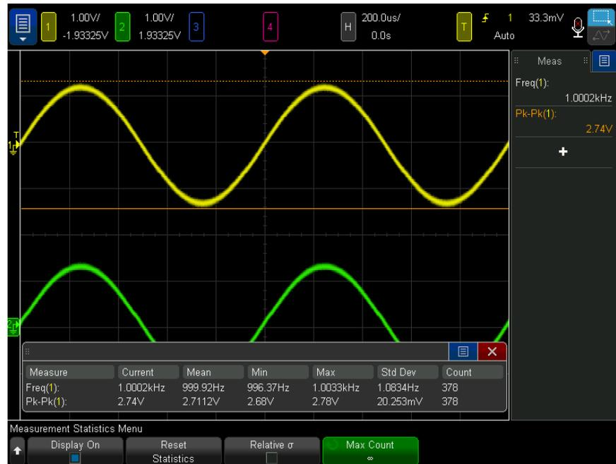
The source channel of the measurement is shown in parenthesis after the measurement name. For example: "**Freq(1)**" indicates a frequency measurement on channel 1.
