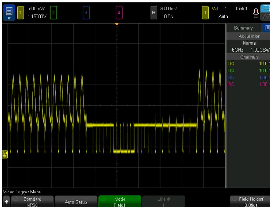
**Figure 31** Triggering on Field 1
