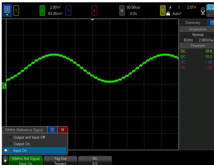
If the externally supplied sample clock signal is lost, a hard unlock will occur. The lock symbol in the upper right part of the display will become an unlocked padlock icon and the oscilloscope will stop acquiring data. The oscilloscope will resume sampling when the externally supplied sample clock becomes stable again.
