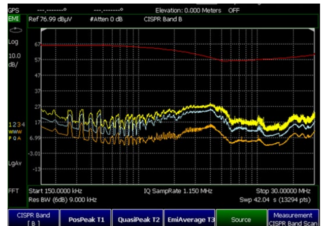
Figure 1. Simultaneous scan with 3 CISPR detectors displayed with a user-defined limit line
