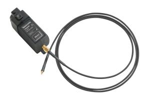
The TPR1000 and TPR4000 probes provide a low noise, large offset range solution for measurement of ripple on DC power rails ranging from -60 to +60 VDC. Tektronix's power rail probes offer industry leading low noise and high offset range required to measure AC ripple between 200  $V_{\text{D-D}}$  and 800 mV<sub>D-D</sub> at up to 4 GHz.
