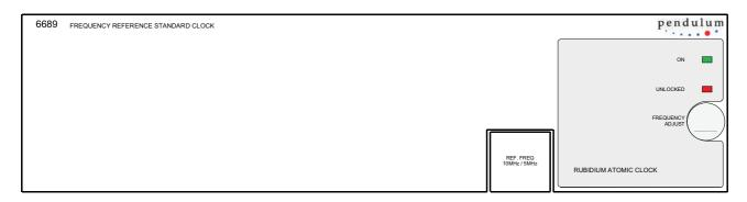
Front panel of 6689. The ON indicator shows when power is connected. The UNLOCK indicator warns when the output frequency is not yet locked to the rubidium element. The adjustment potentiometer is located under the calibration seal
