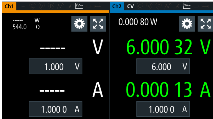
Figure 6-3: Output of Ch2 in CV mode
