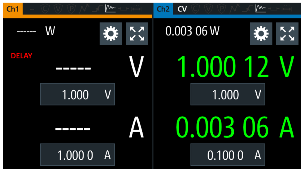
Figure 6-10: Delay text at channel display area
