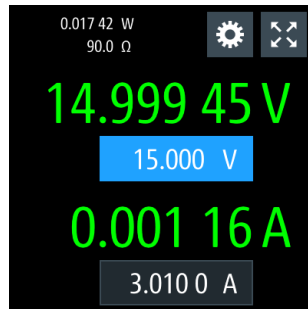
Figure 6-2: Voltage and current settings in the instrument
