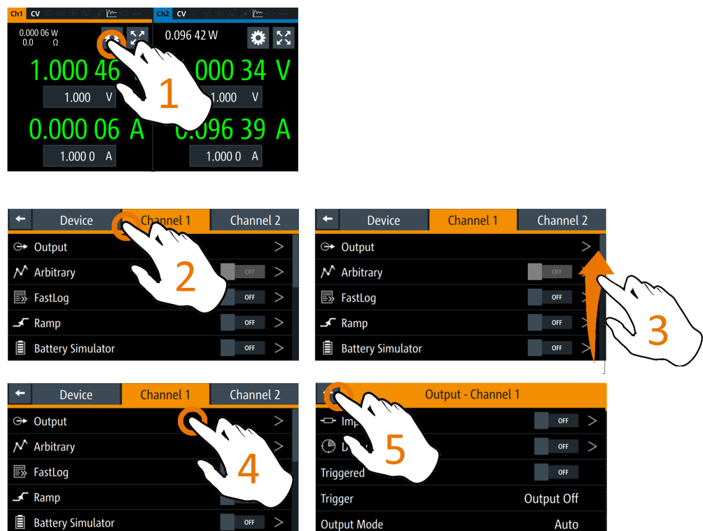
Figure 5-4: Navigation on home window > device/channel menu window
