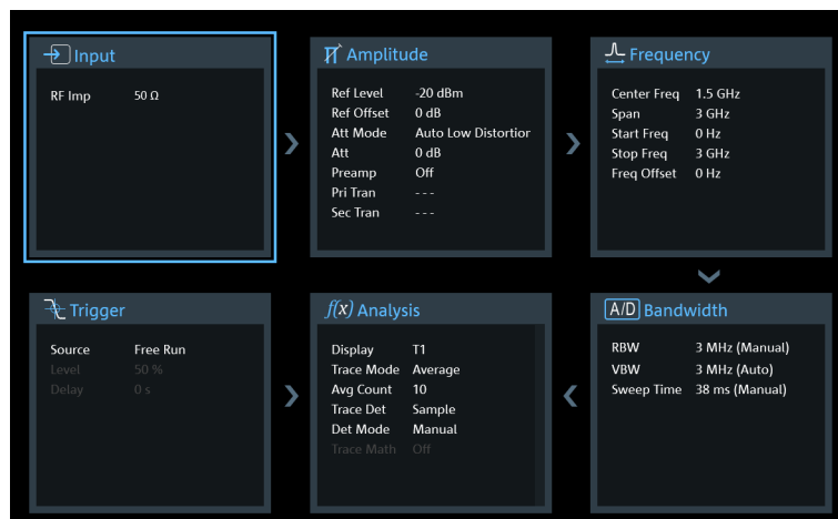
Figure 14-1: Configuration overview in the spectrum application
