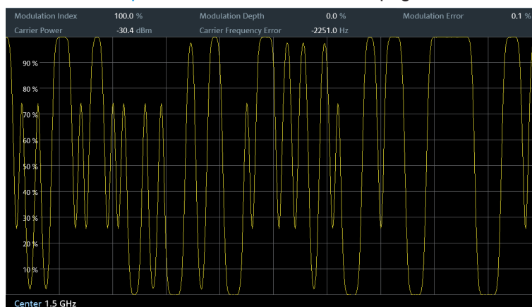
Figure 17-4: Modulation depth of a 2ASK signal
