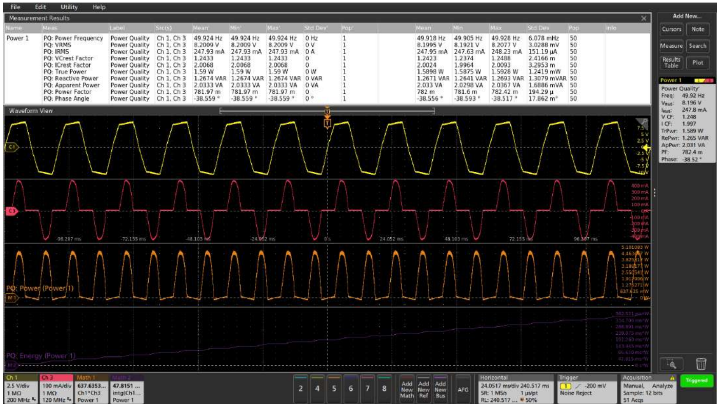
Power Quality measurements deliver information in multiple formats. Numerical results (upper right), tables (upper), and instantaneous power waveform and energy plots (lower).
