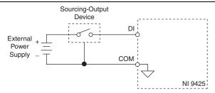
The NI 9425E channel registers as ON when the sourcing-output device applies a voltage or drives a current that is in the input ON range to the DI pin. The channel registers as OFF when the device applies a voltage or drives a current that is in the input OFF range to the DI pin. If no device is connected to the DI pin, the channel
