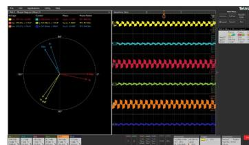
Debug motor drive designs by viewing the drive input/output voltage and current signals in the time domain simultaneously with the phasor diagram.
