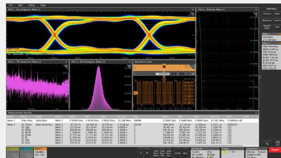
Jitter and timing analysis: Extended analysis functions such as eye diagrams and jitter analysis are optional.
