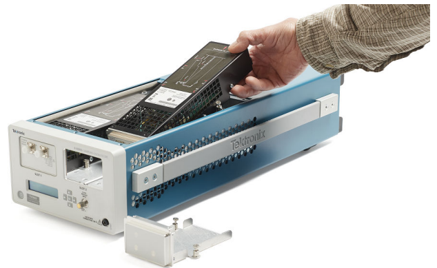
Plugging TSO8C18 module into TSO820 mainframe.
