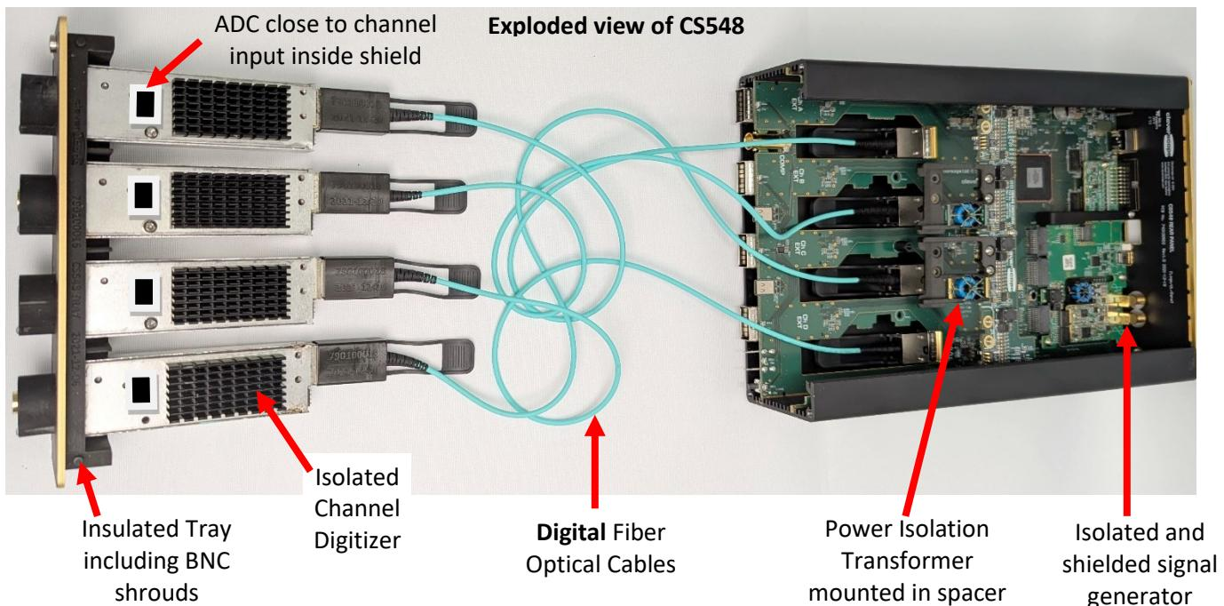
We have built the CS548 with the assumption that the UUT is powered by a line to neutral mains voltage <600 V<sub>AC</sub> and includes secondary circuit working voltages of <2 kV<sub>DC</sub> or V<sub>AC-PEAK</sub>. This is measurement category III. These standards apply:
