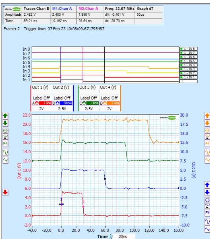
Here 4 pulses have been defined, and output via a CS1302. Outputs 1-3 are mirrored as Inputs 1-3. Input 4, which is a CS1302 input, is physically measuring Output 4. Pulses as short as 17ns can be generated using the CS1302. The incremental step resolution is 4.3 ns. These pulses are 30, 60, 90 and 120 ns long.
