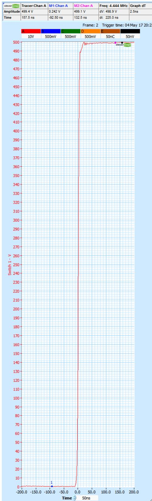
This trace shows the transition measured using a 100x probe. The display pixel resolution masks the actual channel resolution, shown here at 1 V/div:
