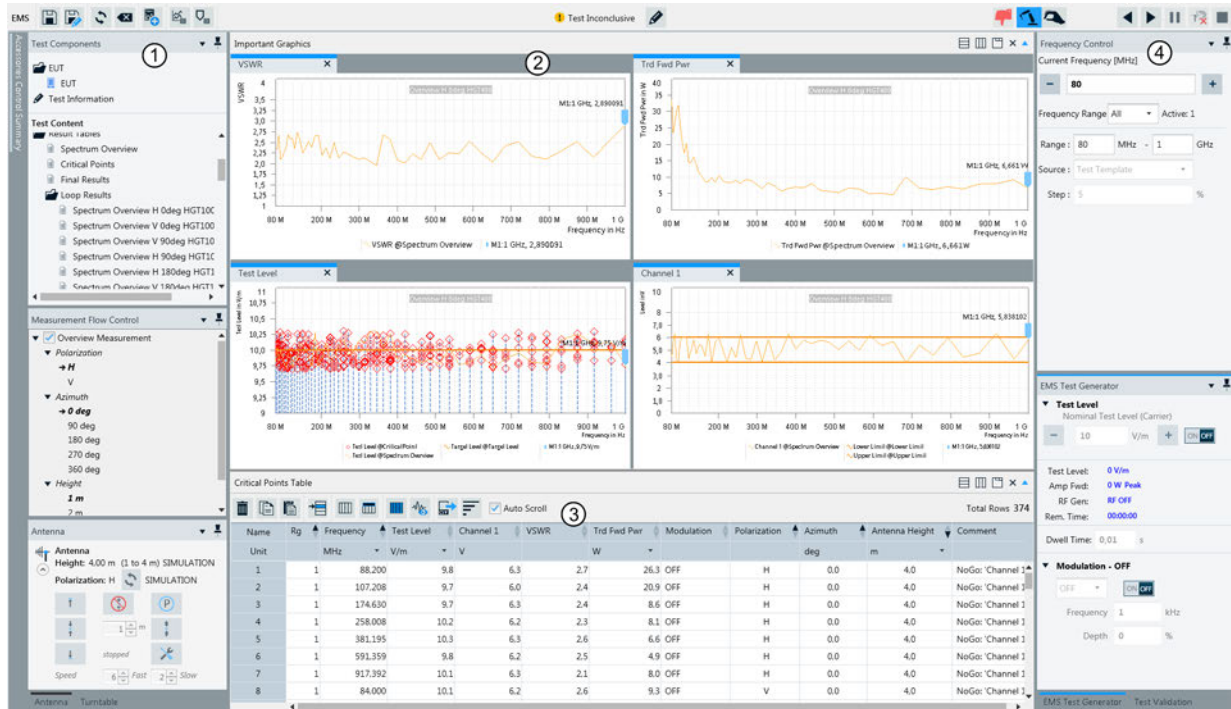
Figure 3-9: Example of a test window
