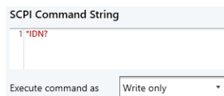
Figure 4-168: Example for the Identification command of a generic amplifier (here: from manufacturer "Bonn", which is shown as an editable Required Substring in Answer)
